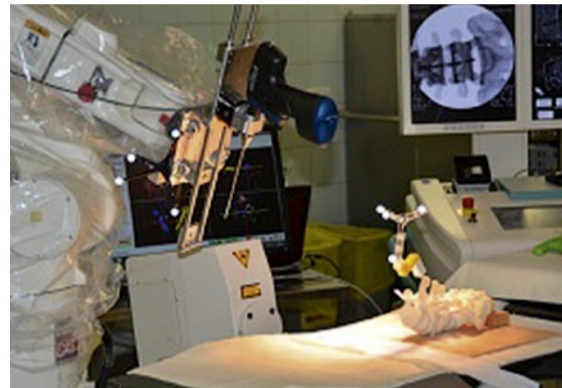
An assistance system for minimally invasive spinal surgery: Robot-assisted positioning of screws on a model of the lumbar vertebrae at the Research Project Centre for Sensor Systems (ZE5S), University of Siegen and Neurosurgery Karlsruhe
